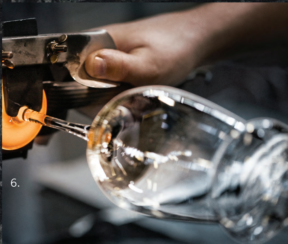
6. The glass moves on to the deputy master blower, who adds more glass and, using a clapper, fashions the foot of the glass.
