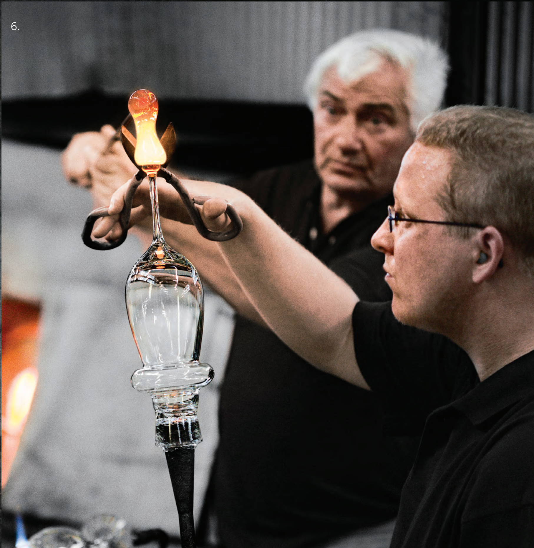
6. The glass moves on to the deputy master blower, who adds more glass and, using a clapper, fashions the foot of the glass.
