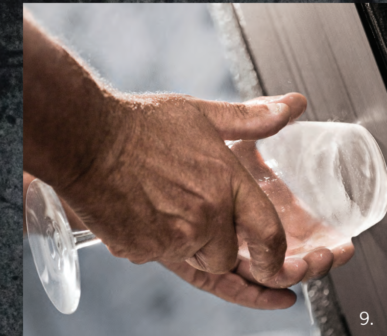
9. Then the sharp edge is carefully ground and polished. Finally, the edge of the bowl is heated until it melts and is softly rounded.
