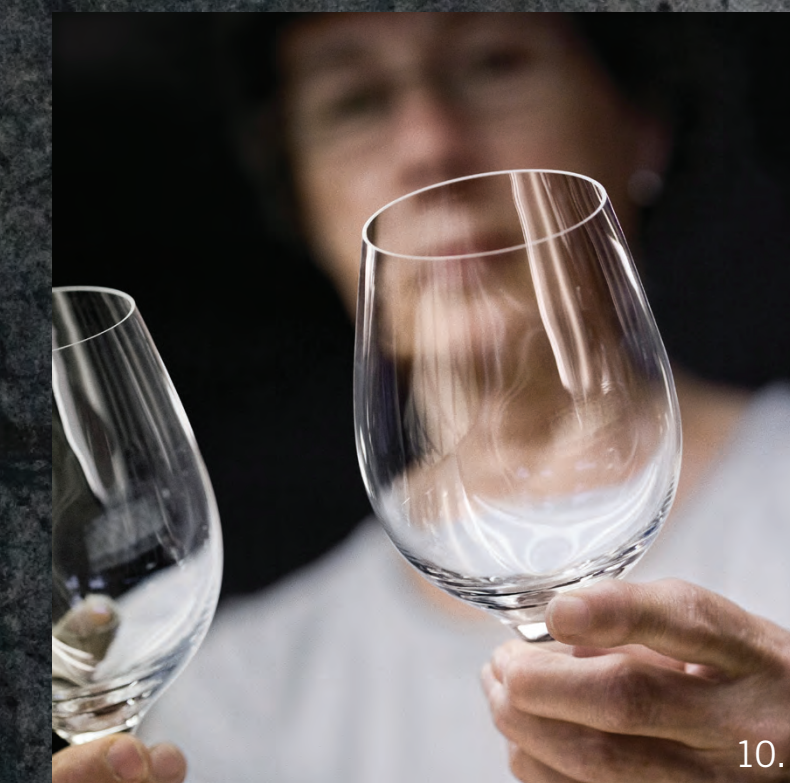
10. When ready, the glass undergoes final inspection and sorting. Finally, as a guarantee of quality, the finished glass is marked with the Orrefors shield: one is sand-blasted into the bottom of the glass, while a silver label is applied to the foot.
