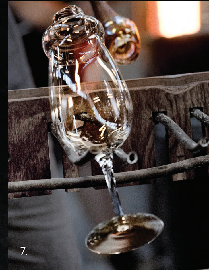
7. The assistant knocks the glass off the blowpipe using a special holder known as a carry-in-fork. The glass is then fetched by a carrier, who places it in a lehr, where it is slowly cooled. After cooling, an initial quality assurance check is carried out by a sorter. If the glass is deemed to comply with Orrefors' stringent quality standards, it is sent for further processing.
